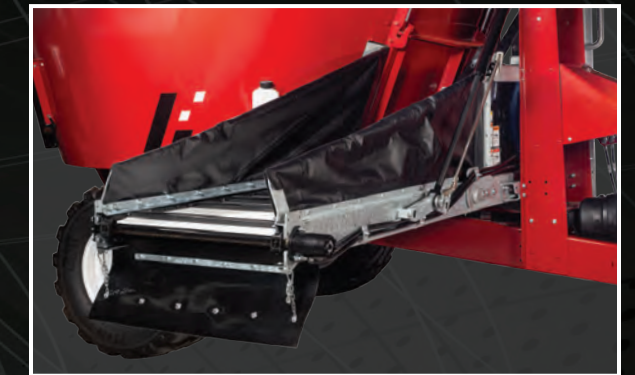
LONG WING CONVEYOR – 72": LEFT OR RIGHT DISCHARGE
